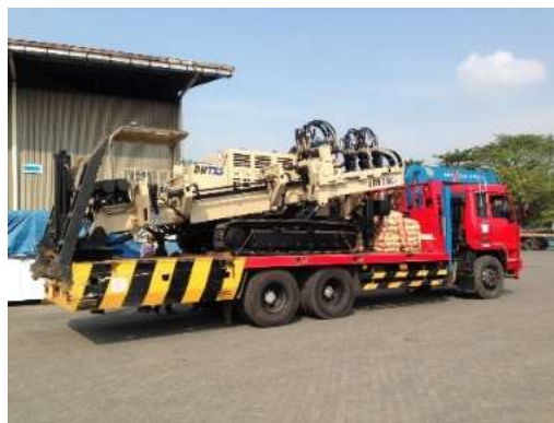
Gambar 1 Alat Horizontal Directional Drilling
