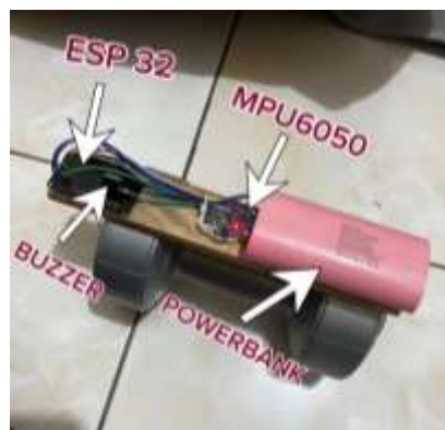
Gambar 1. Smart Dumbbell Berbasis IoT
