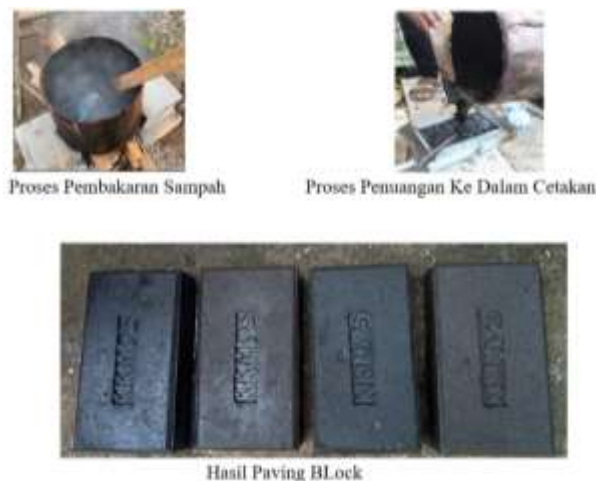
Gambar 1 Pengolahan Paving Block Bahan Baku Sampah
