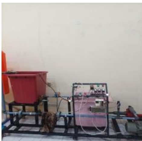
Figure 5. SCADA-based level and pressure control plant prototype
