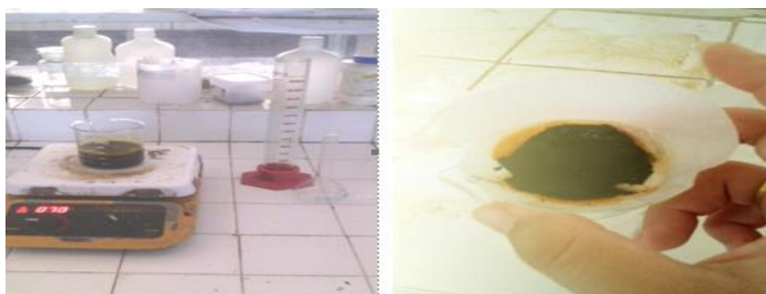
Figure 3. Magnetite Fe 3 O 4 synthesis process coprecipitation method
