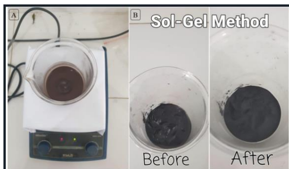
Figure 4. Synthesis process of magnetite Fe 3 O 4 nanoparticles using the sol-gel method
